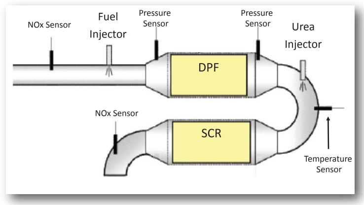
referred to as the SCR for Selective Catalyst Reduction, but it is where the reactions to convert NOx to nitrogen and water take place.
